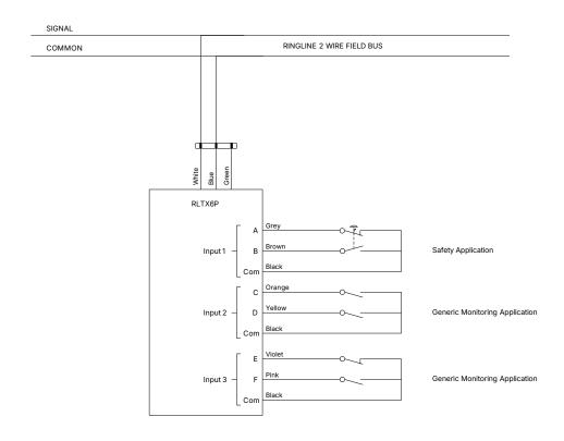
Note: Each set of inputs can independently be used as a Safety or Generic type input
