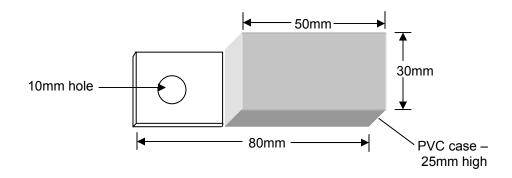
The Ringway Temp7090 is an economical digital temperature-monitoring device with two temperature set points. The device has normally closed interlocks, which open nominally at 70 and 90 degrees Celsius respectively. The device is housed in a PVC enclosure and fully is encapsulated in epoxy resin.
